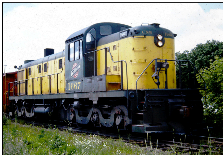
Taken by Phil Rood in 1969, this is a Chicago and Northwestern C&NW diesel taken at the Seventh Day Baptist Church (now Anchor of Hope Church), and is a 1500 horsepower locomotive built by Alco (American Locomotive Company) designated RSD-4. The C&NW ran Alco locomotives on this line, and it therefore came to be identified as the "Alco Line."
